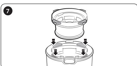
Put the washable micro filter in the dustbin cover by fitting in grooves of the dustbin cover.
