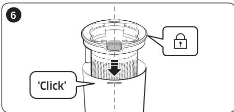
Reassemble the dustbin cover aligning the dustbin release button with the groove of dustbin.
