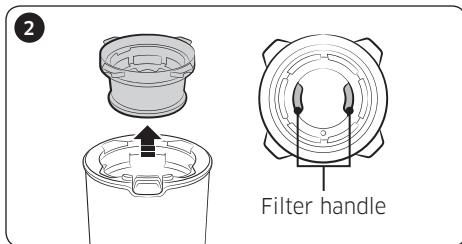
Pull the washable micro filter out by holding the filter handles inside the washable micro filter.
