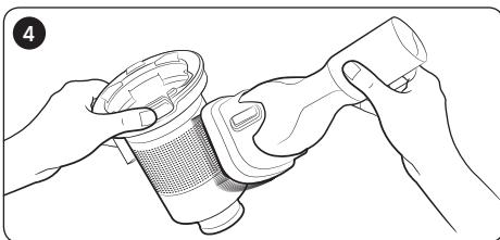
Remove the dust on the metal mesh grille filter with the combination tool.
