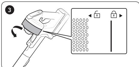
\* When assembling, turn the filter until the line below the lock image is not visible.
